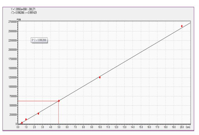
Figure 3: Hydromorphone Calibration Curve (0.5, 1, 2.5, 5, 10, 20ng/mL) R<sup>2</sup>= 0.9982
