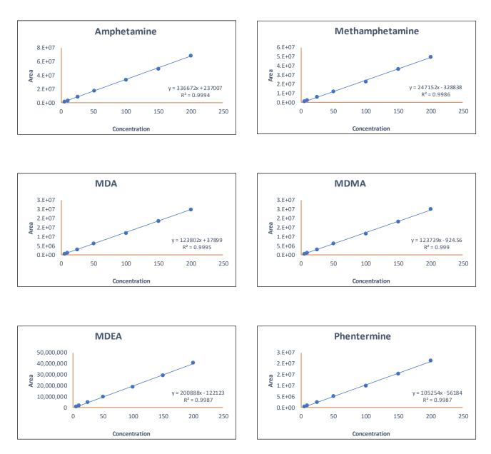
Figure 4. Calibration curve for the six amphetamines (5, 10, 25, 50, 100, 150 & 200 ng/mL).
